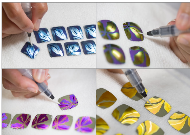
Figure 9: Brush anodizing. Four examples of details being added by brush anodising (photos: Holly Yashi Design Inc.)
