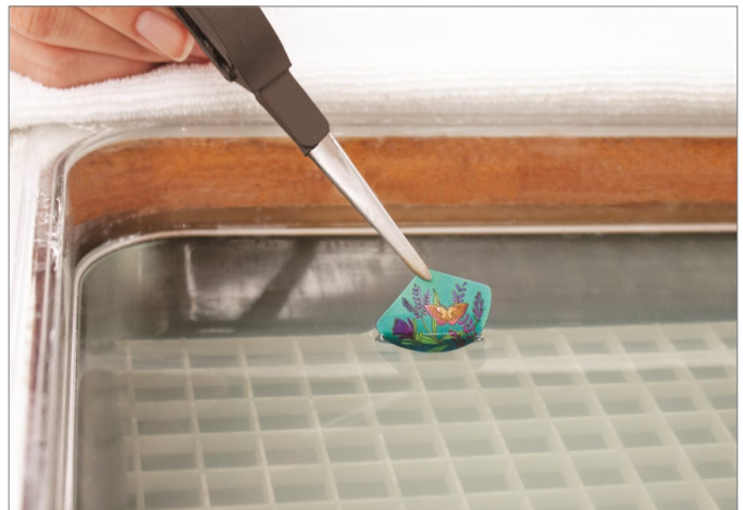
Figure 8: Immersion anodising. A piece of niobium is held by insulated tongs and dipped in electrolyte (photo: Holly Yashi Design Inc.)
